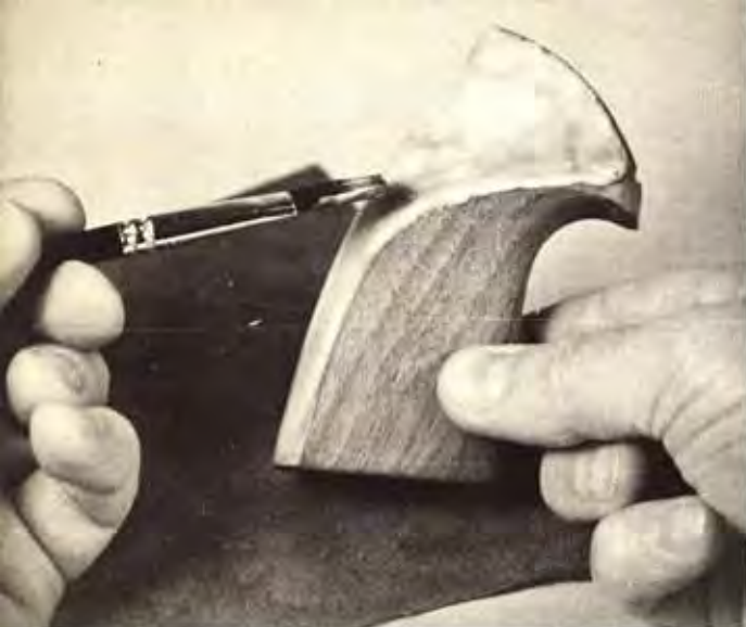
In covering the Dan Wesson, leather is first glued to thumbrest line and around to the flat section on back to avoid any wrinkles.
