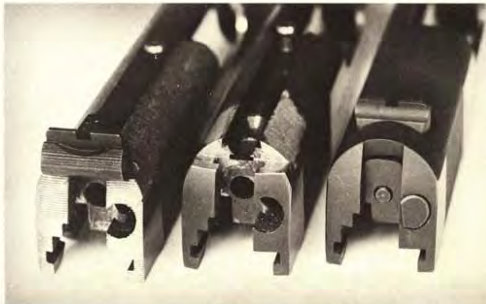
Steps in installing the S&W "K" model rear sight. The commercial slide (right) is milled (center) and completed job is shown at left.
