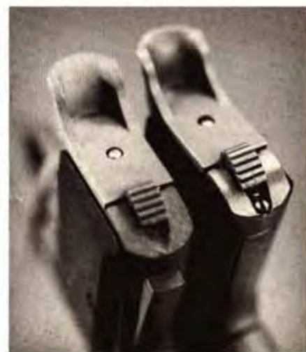
Small screw on altered gun (right) cancels operation of grip safety.
