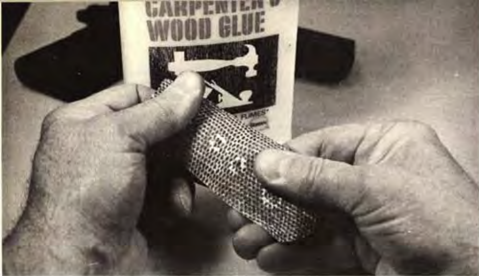
Lizard skin is smoothed over the tacky glue coating on the outer face of the panel. Hard finger pressure is used to obtain a smooth, tight surface.
