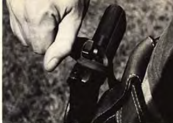
Auto-Flex strap is made of surgical rubber. It holds pistol in place and blocks hammer from firing pin.
