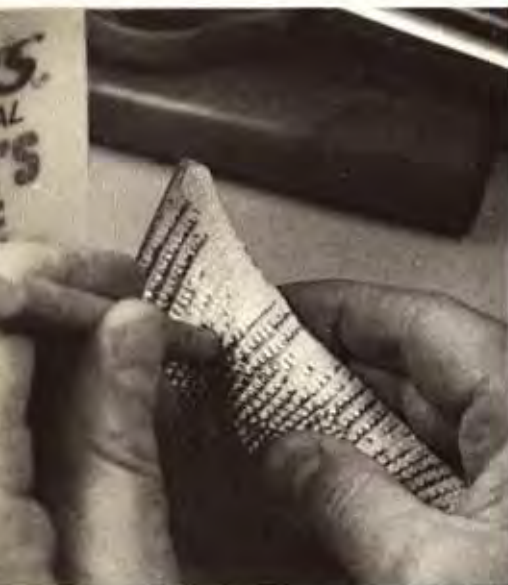
Hide over the screw holes is cut in a star pattern, glue is applied and then pressed into hole with a dowel.
