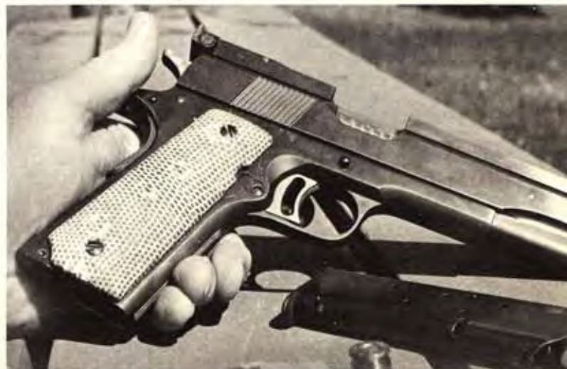
Finished grips on .45 auto are unique and handsome. The rough surface also provides a non-slip handhold.
