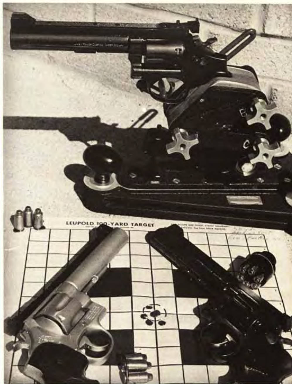
In the Ransom Rest is a PPC gun built on M-19 frame; left is a Douglas barreled .45 ACP on M-25; right is PPC gun on M-13.
