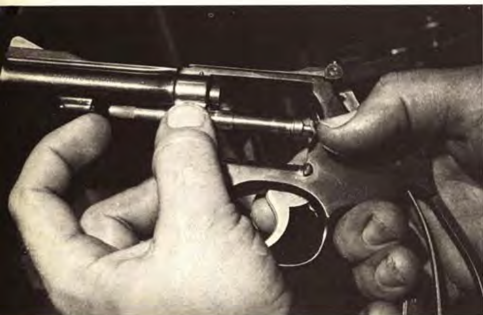
In text, Power explains use of his special tool to determine cylinder line-up characteristics on a M-19.
