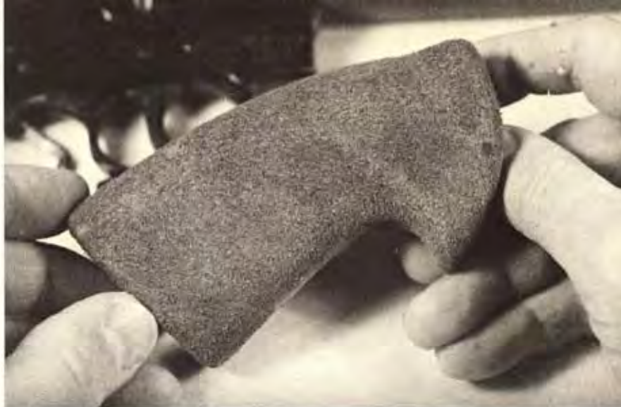
The finished Dan Wesson grip with its suede covering. This provides a soft feeling—but very solid—gripping surface. Shown here the suede is left natural, but it may be sealed.
