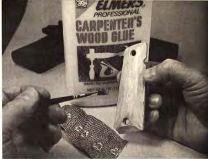
Wood glue is applied to panel and slightly oversize piece of hide is pressed in place.
