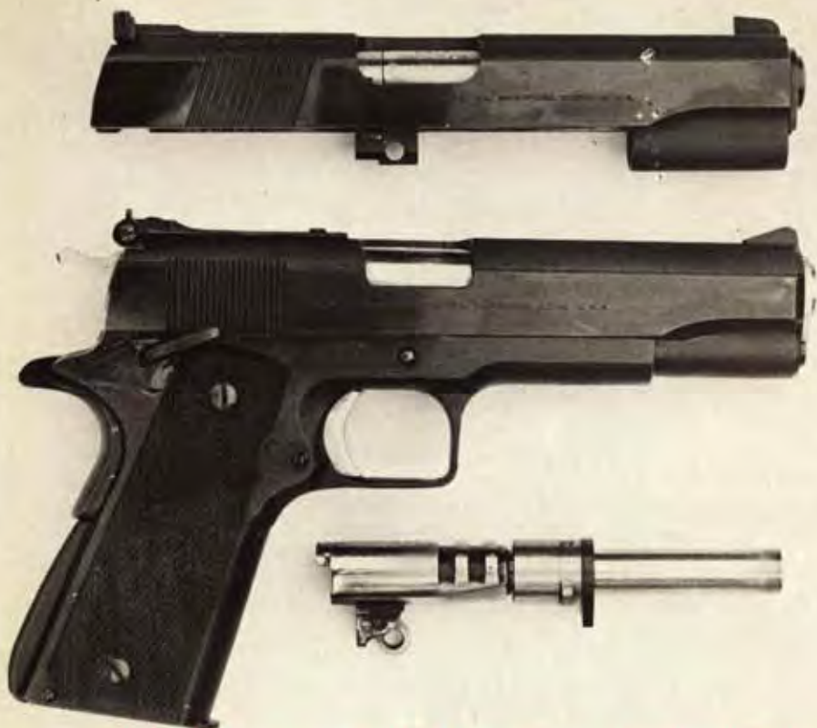
A standard accuracy set up by Swenson. The Government Model is given full house treatment and fitted with a .22 conversion unit and a .38/44 barrel and bushing for multi-purpose use.
