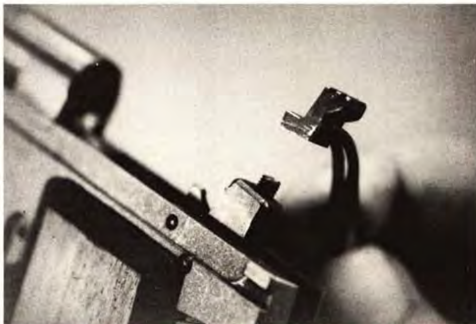
Close-up of the new hammer extension being positioned on the headless screw section which was installed in the top of the hammer.
