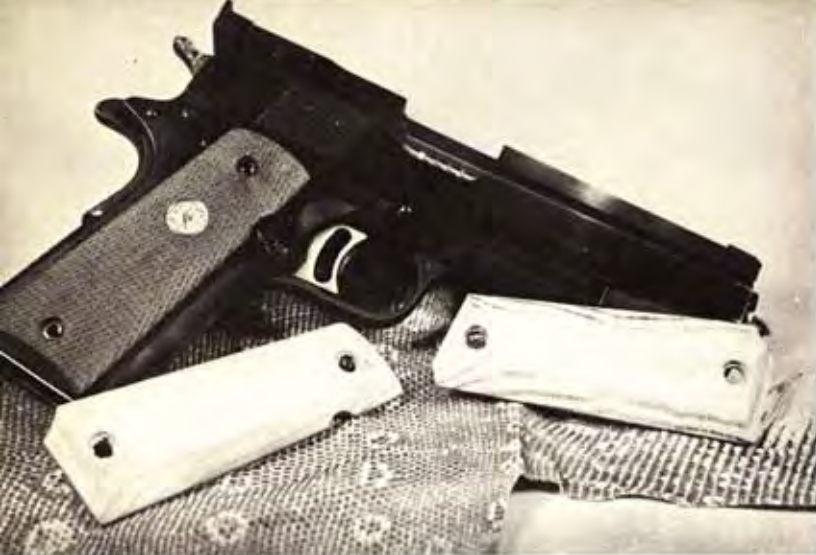
Base for the new grips was made from scrap 1/4-inch hardwood plywood and rough sanded.
