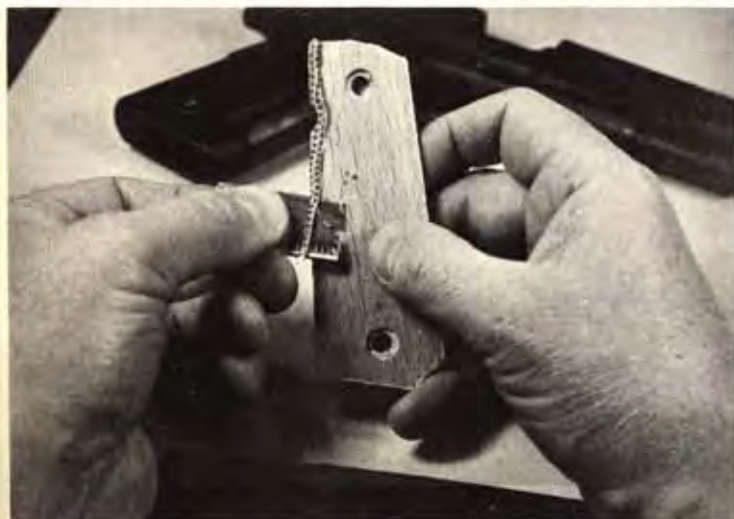
Excess hide is trimmed off of panel back. This is done before glue hardens and excess glue is removed.
