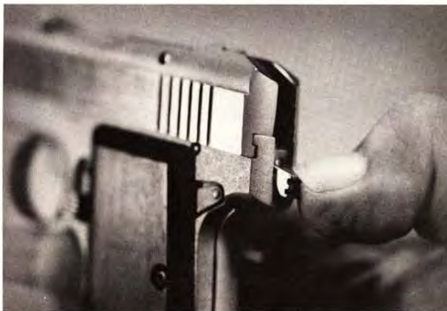
Spur of the new hammer extension comes perilously close to the shooter's hand at full recoil and those with fleshy hands may have some problems.
