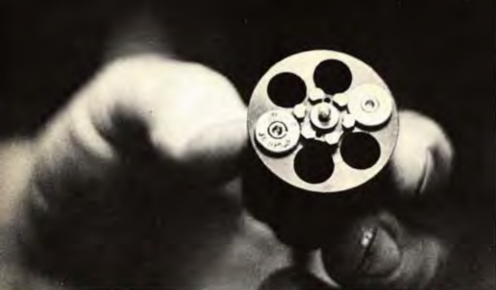
Two strategically placed empty cartridge cases can sharply reduce stress on cylinder components during disassembly, as Power explains in text.
