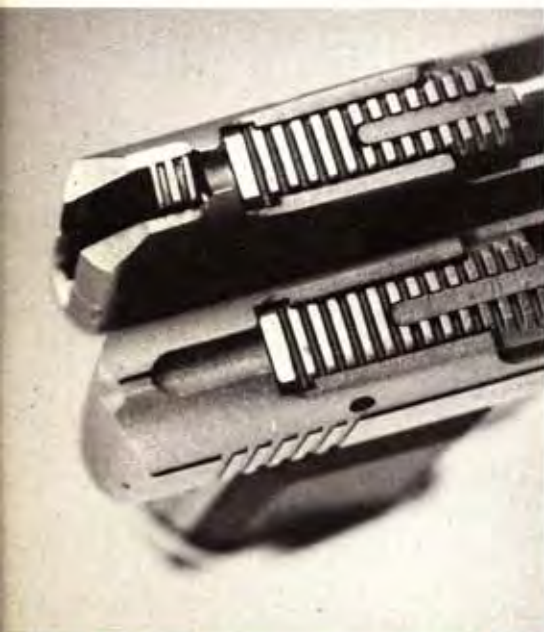
Comparison of the customized OMC with external hammer and unaltered original.
