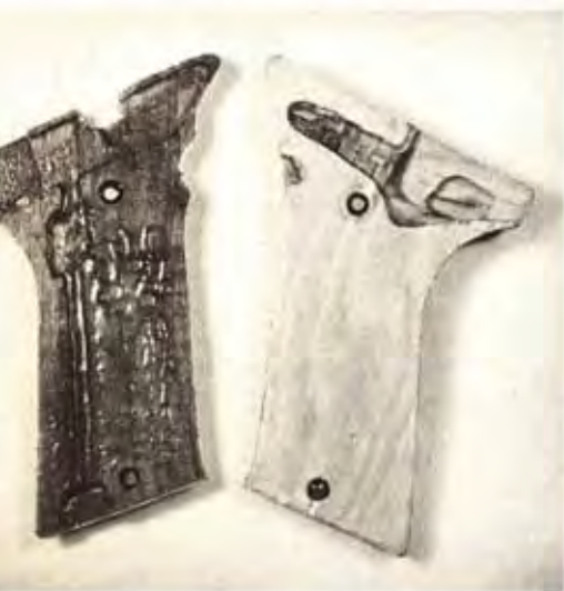
Auto-Mag grips require cuts in the panels and are thus weakened. The wood was hardened with epoxy glue.
