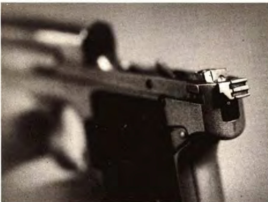
Clearance below hammer in frame allows hammer "whip" during recoil.
