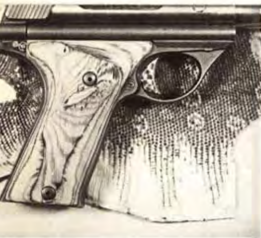
Right hand Auto-Mag grip was made from fir plywood and fitted to the gun before covering with the hide.
