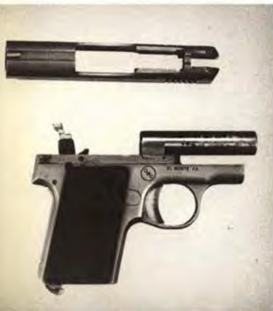
The OMC pistol with slide removed shows the new hammer extension in semi-safety mode.
