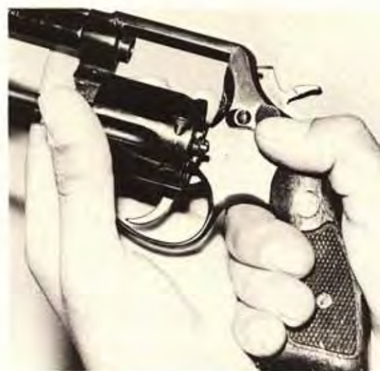
Cylinder latch can still be used to open cylinder, but author had found it possible to move it up to "safe" position accidentally.
